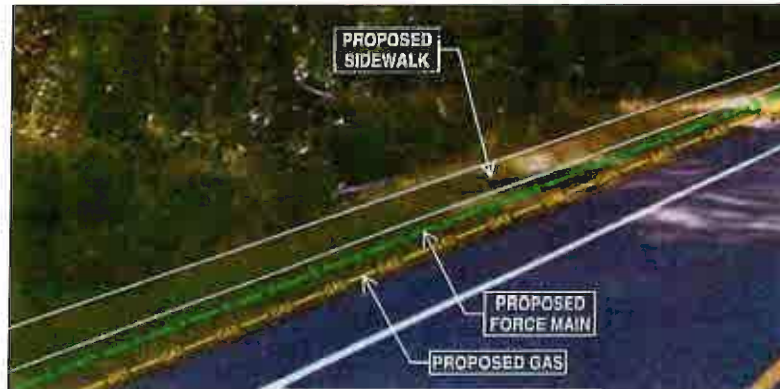
Figure 1 – Schematic location of sidewalk, gas & force main
